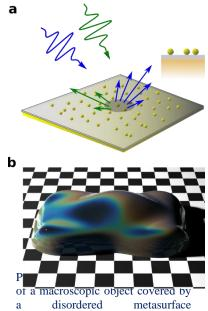
or a macroscopic object covered by a disordered metasurface specifically designed. a. Sketch of the metasurface. b. Appearance obtained by our nano-rendering tool. The appearance of the object drastically changes when moving around the object or changing the light source position.
